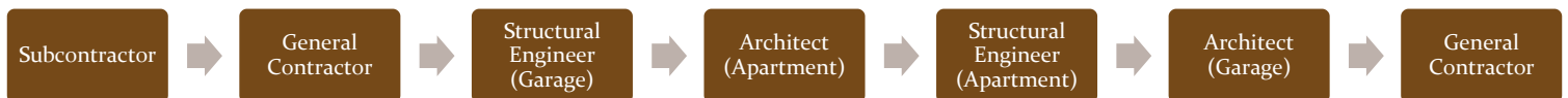
Figure 3: Typical Process of an RFI or Submittal in Octants A, C, and E
